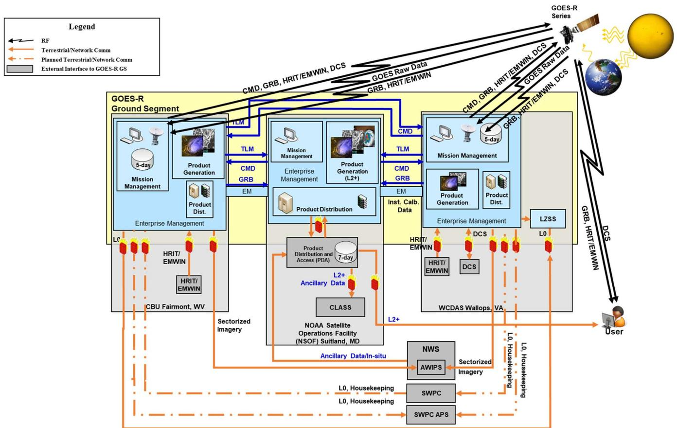
Figure 1: GOES-R Ground Segment Overview (CCR01457, CCR01661, CCR02089, CCR03255, CCR03379, CCR03483)
