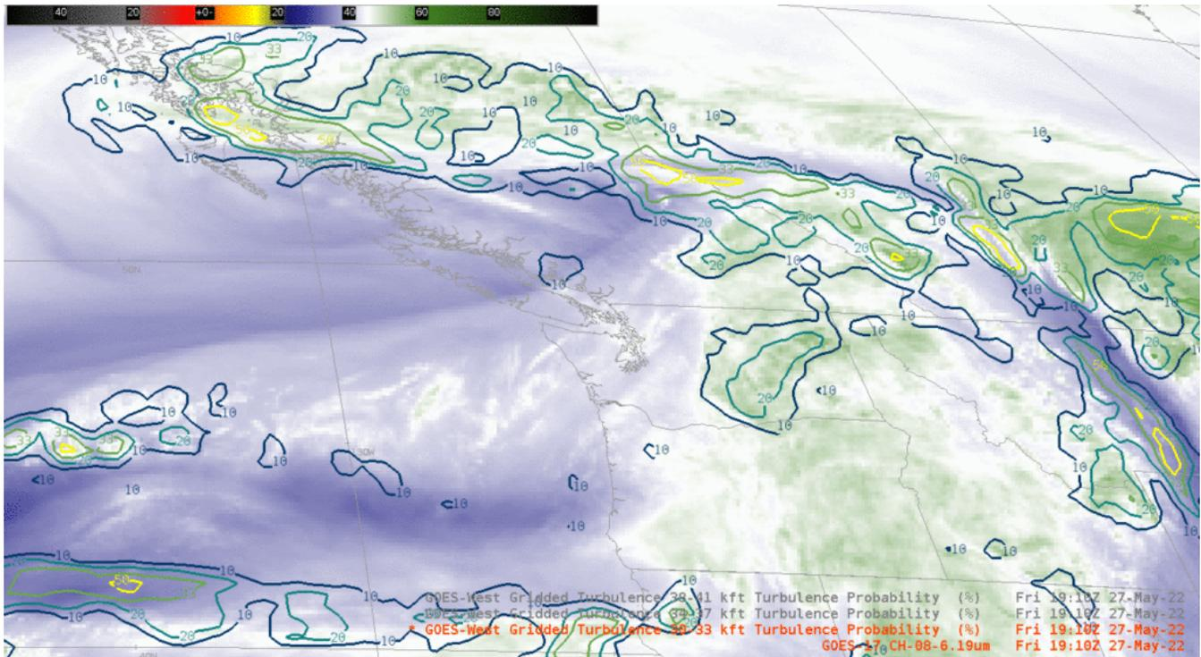
Figure 1. GOES-17 Band 8 (“Low-level water vapor”) Infrared (6.19  $\mu\text{m}$ ) fields, 1910 UTC on 27 May 2022, along with derived Turbulence Probability for 30-33 kft, 34-37 kft, 38-41 kft.
