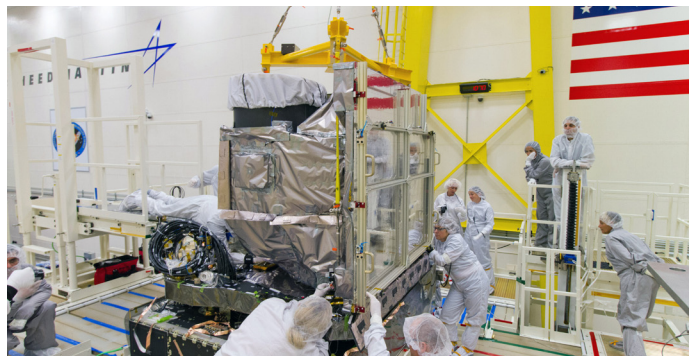
The GOES-R SEISS (upper left), GLM (upper right) and ABI (lower) are installed on the GOES-R spacecraft at Lockheed Martin in Littleton, Colorado. Credit: Lockheed Martin
